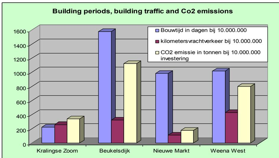
Figure 2. Building period, CO<sub>2</sub> emission and building traffic in four infrastructure projects
